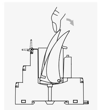
Removing the relay from the socket
