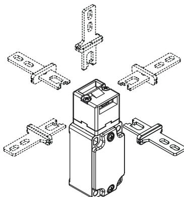
For all switches, the head can be adjusted in 90° steps after removing the two fastening screws. In this way it is possible to actuate the switch from 5 different directions.
