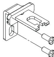
As required by EN ISO 14119, the actuator must be fixed immovably to the door frame. Pan head safety screws with one-way fitting are available for this purpose. With this screw type, the actuators cannot be removed or tampered by using common tools. See accessories on page 310.
