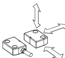
The coded magnetic sensors were designed to be activated by the respective actuator from various directions. The customer therefore enjoys maximum flexibility when positioning devices along the perimeter of the guards.
