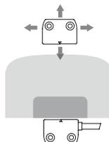
With their built-in features, magnetic sensors have a wide actuation range, making them very well suited for applications with large tolerances or where mechanical properties change over time. In this type of sensor, the actuation distances may vary depending on the shift direction of the actuator in relation to the sensor.
