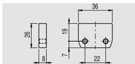
This spacer is placed between the magnetic safety sensors and metal surfaces that can deflect the magnetic field: as a result, the activation and deactivation distances of the sensor remain the same. Because it is made out of a single block of material, it is especially well suited for applications where a high level of cleanliness is required, as any material present in the installation area cannot penetrate and accumulate.
