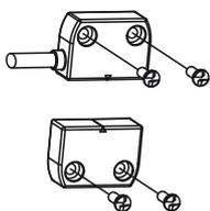
As required by EN ISO 14119, the actuator must be fixed immovably to the door frame. Pan head safety screws with one-way fitting are available for this purpose. With this screw type, the actuators cannot be removed or tampered by using common tools. See accessories on page 310.
