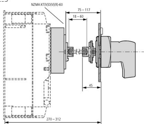
in conjunction with the NZM4-XT(V)D(V)(R) door coupling rotary handle
