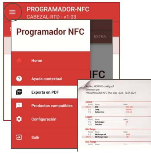
At the top left we find 3 small lines where we can access the app configuration, see the devices compatible with it, access help, exit and something very interesting: generate a PDF file with the device configuration values.
