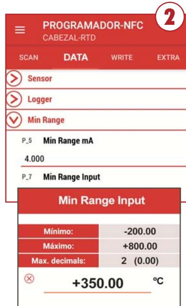
It automatically goes to the DATA tab, where we will see the parameters and can modify them by accessing the drop-down menus (without needing to have the mobile phone near the device).
