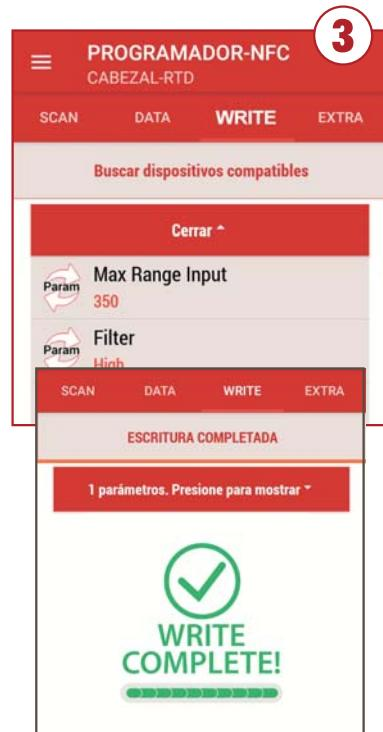
To load the new configuration onto the device, you must access the WRITE tab where you will see the parameters that you have modified. This is where you will again place the mobile phone in contact with the device and wait for the notification that the operation has been completed.
