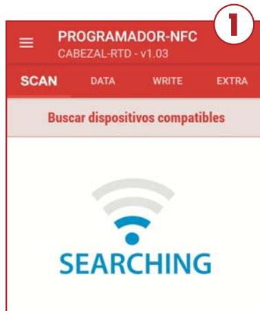
The SCAN tab allows you to read data already recorded on the device. By placing the device in contact with the mobile phone, it will automatically recognize the model.
