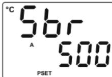
1 - Sensor failure in analogue inputs.
