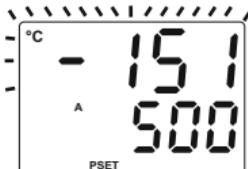
2- If value on top display blinks : If analogue input value is less than minimum value of operating scale  $L_{oL}$ . Value on the top display starts to blink.
